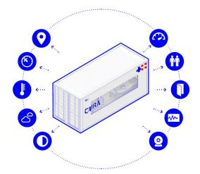
Seluxit and Onomondo's role is to collect data from the so-called CURA pods. The data is telling hospitals about the status of the intensive-care units. Data about air pressure, for example, is critical to make sure the pods' biocontainment technology is working properly. Alerts are sent when filters need to be changed.
